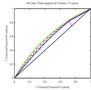
(a) Liquid mole fractions profiles equilibrium column      (b) The McCabe-Thiele diagram between the key components Toluene
